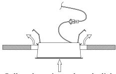
Pull up the spring and put the light into the cut hole.
